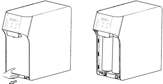
Step 3: Unscrew the old filter and replace with new
