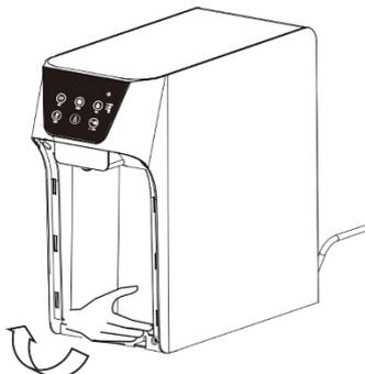
Step 4 : Install back the front panel and tray
